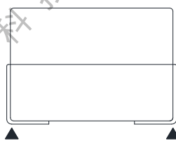
▲ Points used for measuring DCR
