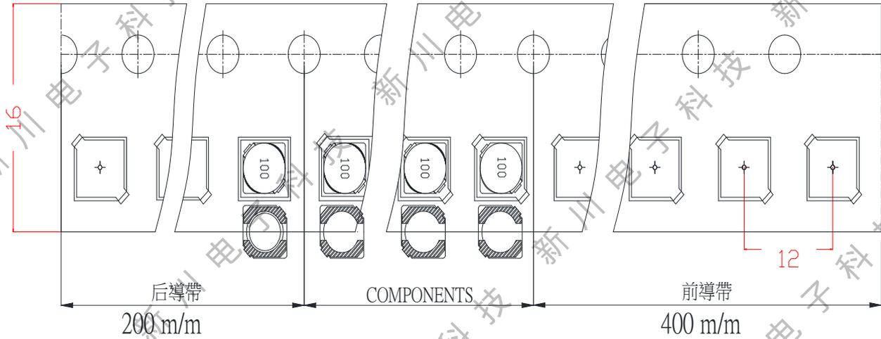
Transparent carrier and cover tape/透明载带和自粘上带
