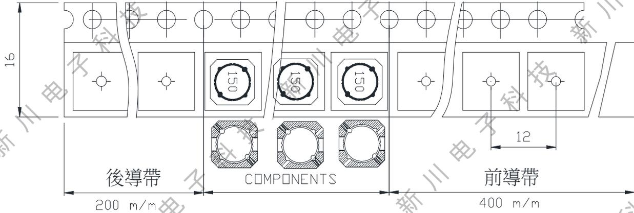
Transparent carrier and cover tape/透明载带和自粘上带
